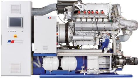
CHP plant with type 12V 400 biogas engine. The compact cogeneration module from MTU Onsite Energy is available with 6 and 12-cylinder Series 400 biogas engines. It produces 120 to 400 kW of electric energy and 160 to max. 540 kW of thermal energy.
