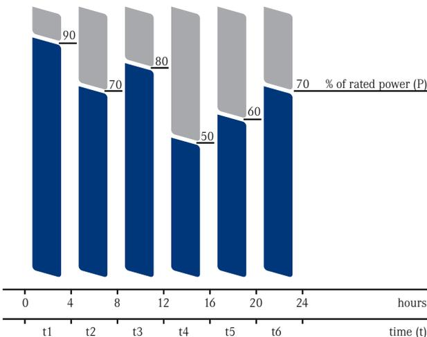
$$ALF = \frac{(P_1 \times t_1) + (P_2 \times t_2) + (P_3 \times t_3) + (P_4 \times t_4) + (P_5 \times t_5) + (P_6 \times t_6)}{t_1 + t_2 + t_3 + t_4 + t_5 + t_6}$$
