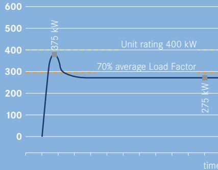
**Scenario 3.** 350 kW generator set, 79% Load Factor, 25 HP motors (6) *soft-started* with 150 kW resistive loads in same step.
