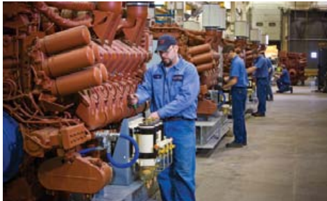
MTU Onsite Energy generator sets for APR Energy's Peru project feature the advanced MTU Series 4000 diesel engines.
