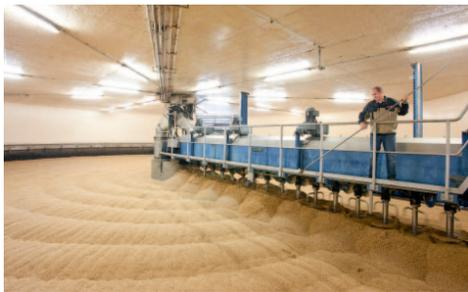
The barley is first steeped in water in large vats until it has a water content of 45 per cent. It is then transferred to the so-called germination or malting chambers, where it is allowed to germinate for a period of six days.
