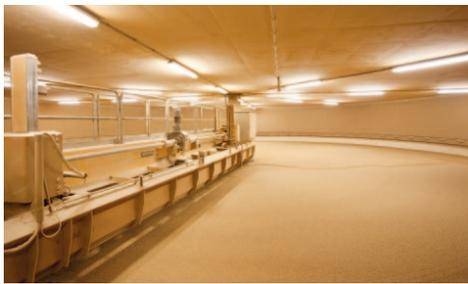
The germinated barley is now allowed to dry again in so-called drying kilns at temperatures of up to 85 degrees Celsius (185 °F). Part of the heat is supplied by the two natural gas-fired CHP plants of MTU Onsite Energy.
